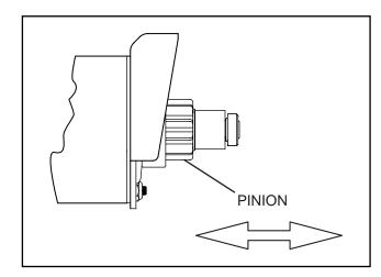
Figure 13. Check Pinion Gear Operation (Single Cylinder)
